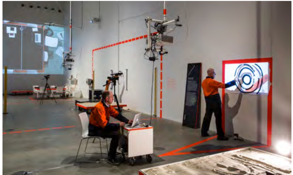
Fig. 3: The feedback system, robot perception via camera and visual information run through software to set parameters for Ela's work-space and work task.
