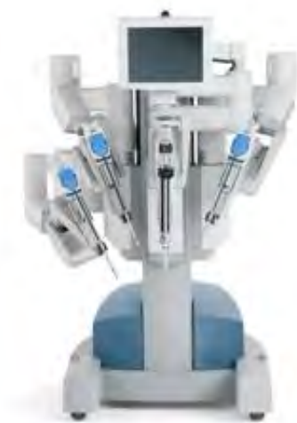
Fig. 4. da Vinci TM surgical cart. The robotic arms contain the endoscopic camera and a range of surgical instruments. ©2007 Intuitive Surgical, Inc.
